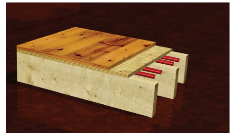
Plywood over joists
