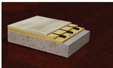
Radiant Heat Tubes In Plywood
